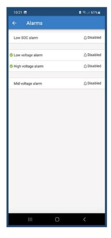
Acoustic alarms are integrated in the BMS in EX-S5. We therefore recommend not to activate the alarms in the VE system.
