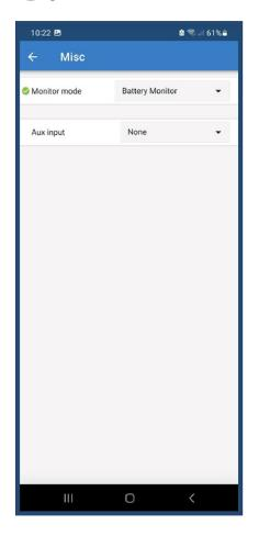
For an overview of the SoC (State of Charge) it is necessary to select the "Battery monitor" mode
