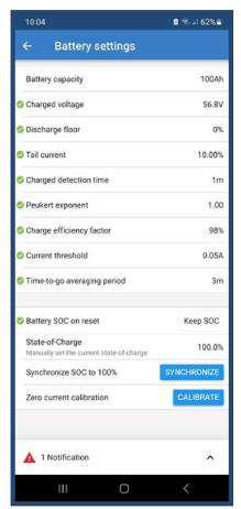
For the most frequent recalibration of the SoC to 100% we recommend:
